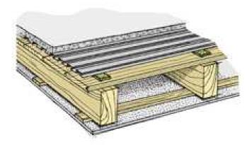
The LEWIS® Dovetailed metal decking is applied at right angles to the beams. Using LEWIS® Rockwool side strips, the LEWIS® sheet floor is kept free from the rising work around. A layer of 34 mm flowing screed is applied onto the Dovetailed metal sheeting. Underneath the dovetailed metal sheet floor, a 12.5 mm thick fibreglass-reinforced plaster board ceiling will suffice. This construction realises a performance of airborne sound Rw 55 and impact sound Ln 49.
