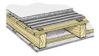
LEWIS® sound-insulating support strips are applied on the existing T&G timber boards or directly on the wooden beams. LEWIS® profiled metal decking is applied onto the resilient strips. Peripheral connection points and conduits are closed off with LEWIS® Rockwool side strips. A layer of 34 mm flowing screed is applied onto the LEWIS® metal decking. The total finished floor thickness applied onto the existing construction is only 65 mm (15 mm resilient strips, 16 mm
